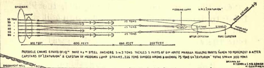
the bow of a tank steamer, and from two "lumps." These were filled and hove down at low water, and pumped out during the operations as the tide rose. (See Plate 2.) Air was pumped in by the destroyer *Handy*, and the water in the upper compartments of the vessel thus forced down to the level marked X on Plate 1, materially assisted.
